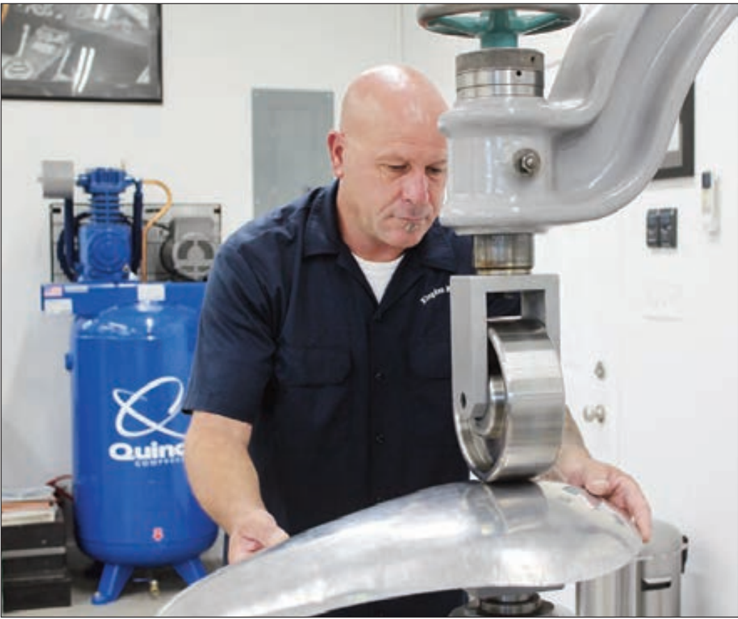
Kevin Masson shapes metal with an English wheel at his shop in Hampton. Masson, originally from Great Britain, moved to the area after working in California for several years.
